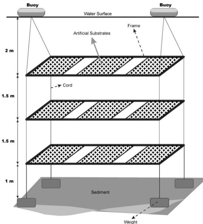
**Figure 2:** Arrangement of artificial substrates at each site for larval chironomid collection.
